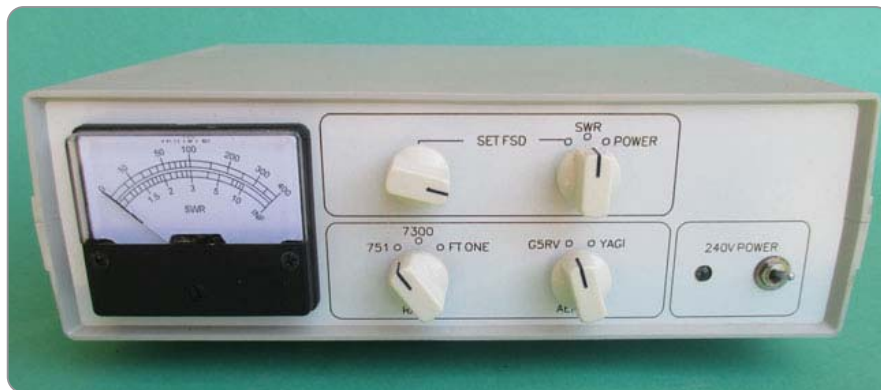
Photo 1: I housed my antenna switch project in an ABS plastic case, 260 x 190 x 80 mm (width, depth, height). I replaced the front and rear panels with 3 mm-thick melamine coated MDF to suit this project. Either operator at this station can select any of three transceivers to connect to either the G5RV multi-band HF antenna, or the Yagi HF beam. Domestic bliss prevails!
