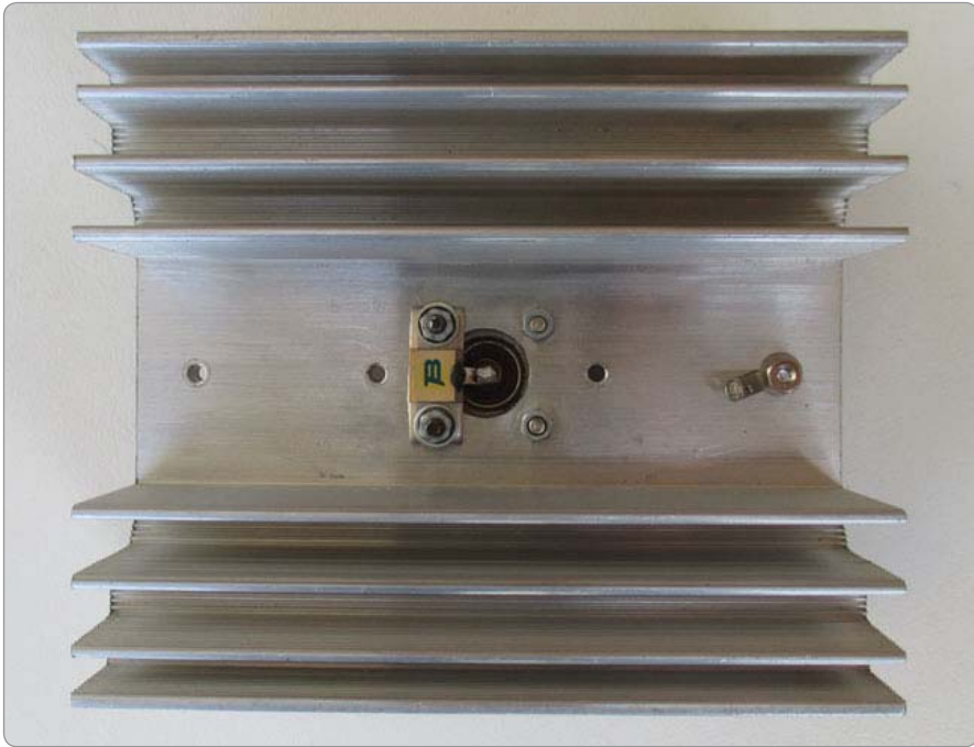
Photo 2: A heatsink, a coax socket and a thin-film resistor – it's simple, alright.
