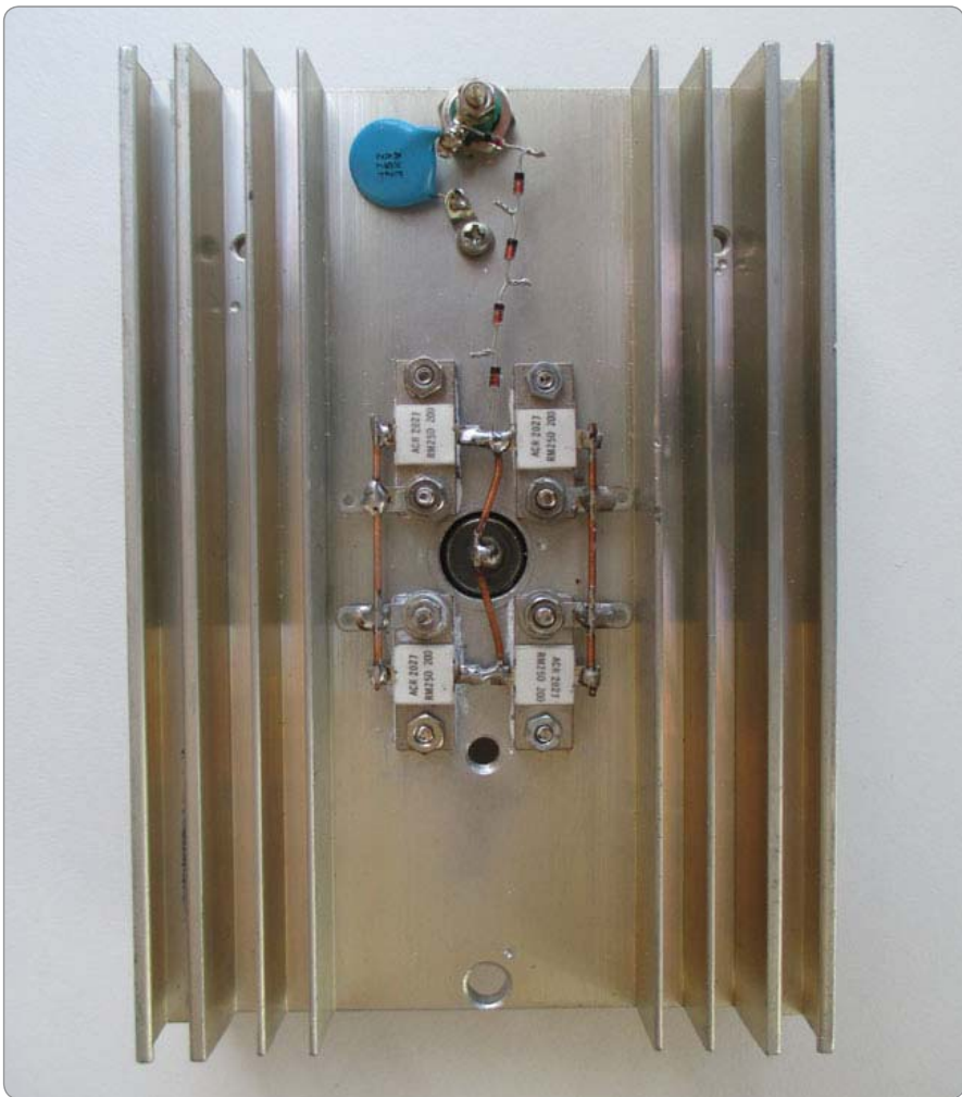
Photo 3: Multiple resistors in series/parallel arrangements enable high power rated dummy loads. The addition of a diode envelope detector, as per Figure 1, enables voltage measurement related to power, as per Table 1.
